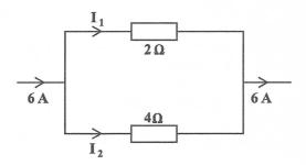
53. Using the information given in the circuit diagram, which pair of values of  $I_1$  and  $I_2$  is correct?
