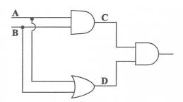
**52.** What is the output at **C** and **D** when an input of 0 0 is made at **A** and **B**?
